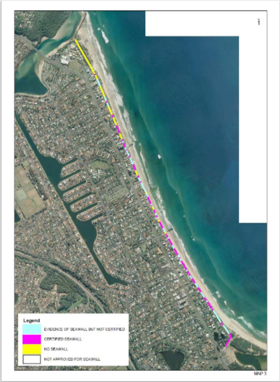
Figure 10 Status of the Seawall at Palm Beach (Source: GCCC, 2012)
