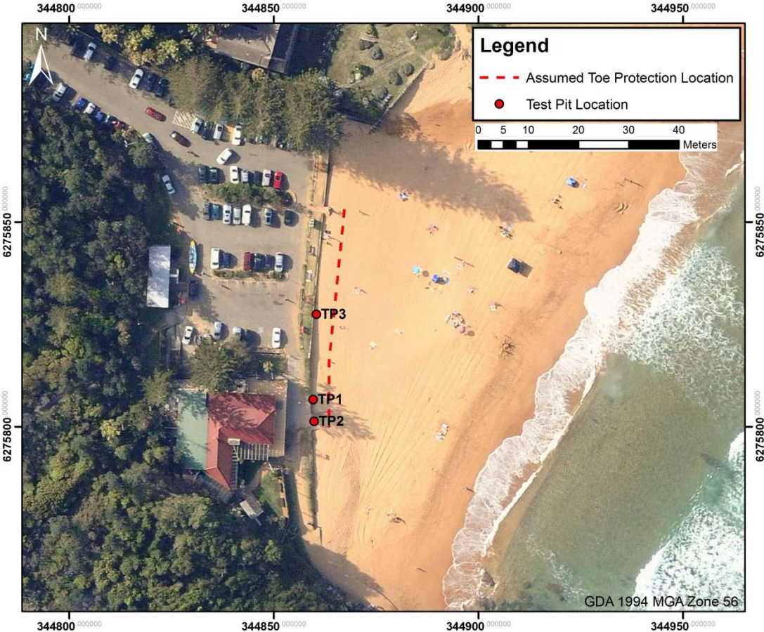
Figure 2.9 Location of Test Pits in Front of Bilgola SLSC Seawall
