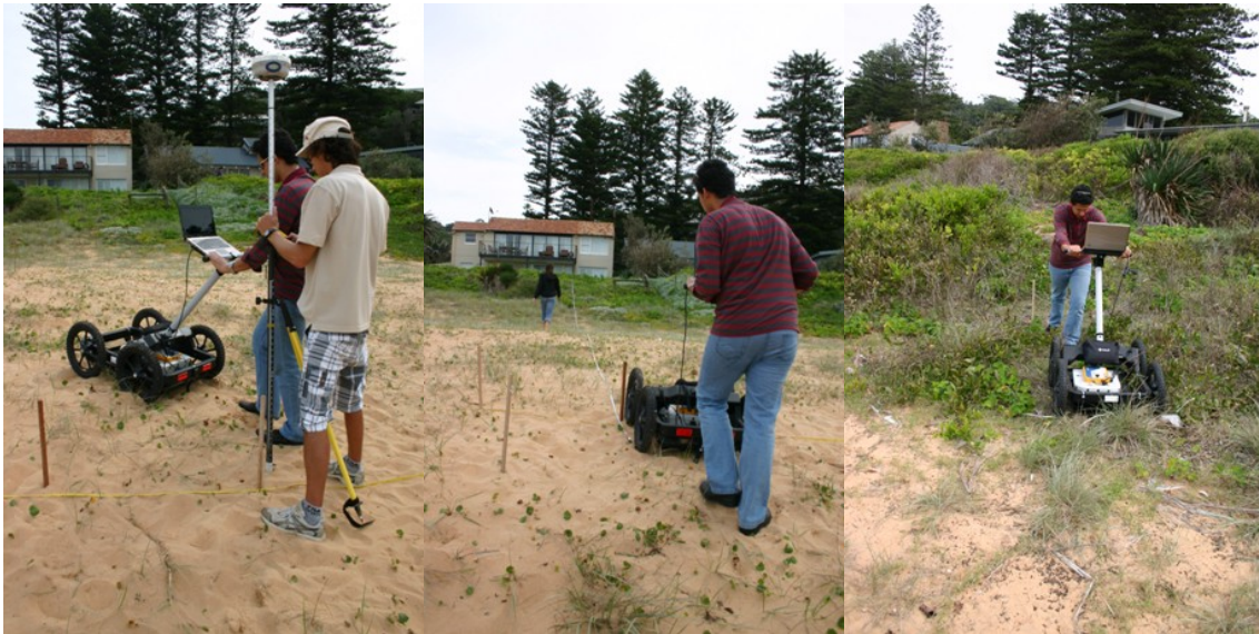
Figure 2.4 Photos of GPR Survey and RTK-GPS Survey
