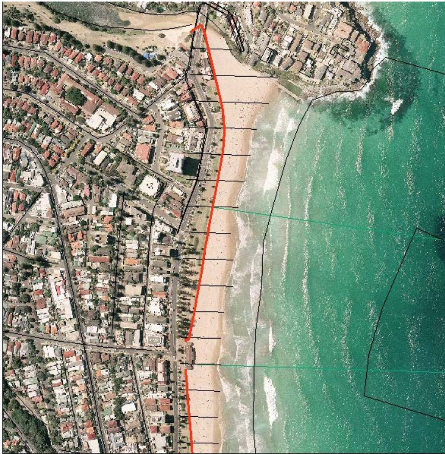
Figure 10 Photogrammetry data for Queenscliff, with resulting shore-normal cross-sections
