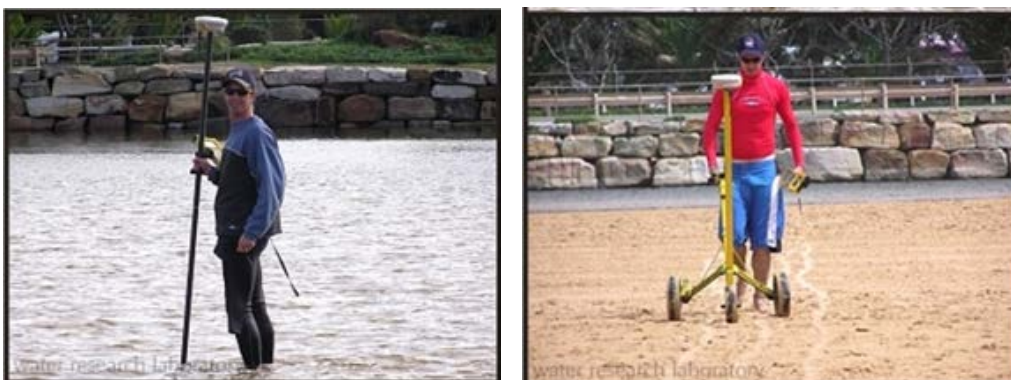
Figure 13 Real Time Kinematic Differential GPS (RTK-GPS) mounted on a survey pole and a three-wheeled cart
